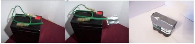
Bare terminals on sealed lead acid batteries can also be a short circuit hazard.
