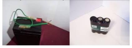
Cut off wire leads flush or cover leads and or pressure contacts with tape or some other non-conductive material to prevent short circuit hazards.
