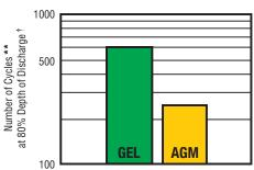
Gel Cycle Life and AGM Cycle Life vs Depth of Discharge at +25°C (77°F) based on BCI 2-hour Capacity
