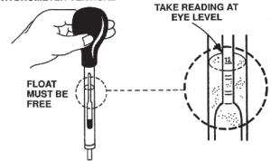
The correct hydrometer reading corresponds to an imaginary line drawn across the side of the barrel at the lowest level of the electrolyte. If the hydrometer has to be removed from the vent hole, pinch the nozzle tightly or place a gloved finger against the opening to prevent dripping.
