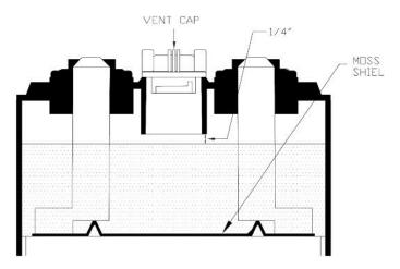
If a large amount of liquid is required to raise the level, the cell jar may be damaged. Inspect the packing material under the tray for signs of leakage. All damaged components should be inspected by your East Penn agent or representative.
