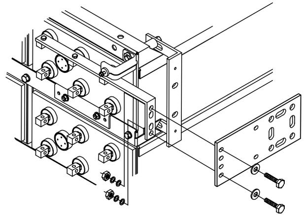
7. After all parts are installed and alignment is confirmed, safety shield bracket hardware should be tightened, but not torqued. All remaining hardware should be torqued. Consult "Hardware Torque Requirements" (pg b.4) for proper torque values.
