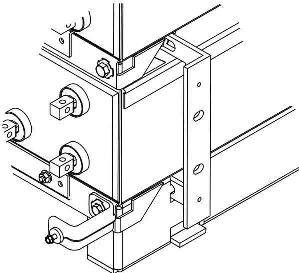
4. Install side terminal connector to battery posts using 1/4-20 bolts. Bolts should be installed loosely for future adjustments.
