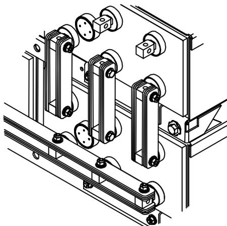
6. Some installations require a vertical “C” connector. This “C” connector is limited to a 2CU connector package. Consult below for proper installation for particular cell type being installed.
