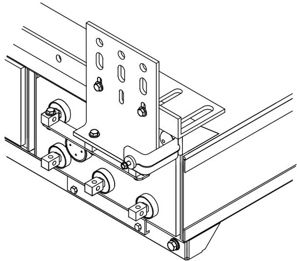
4. Attach terminal plate to terminal plate bracket. Note position of terminal plate. Terminal plate bracket may have to be moved in order to be flush with the terminal plate.
