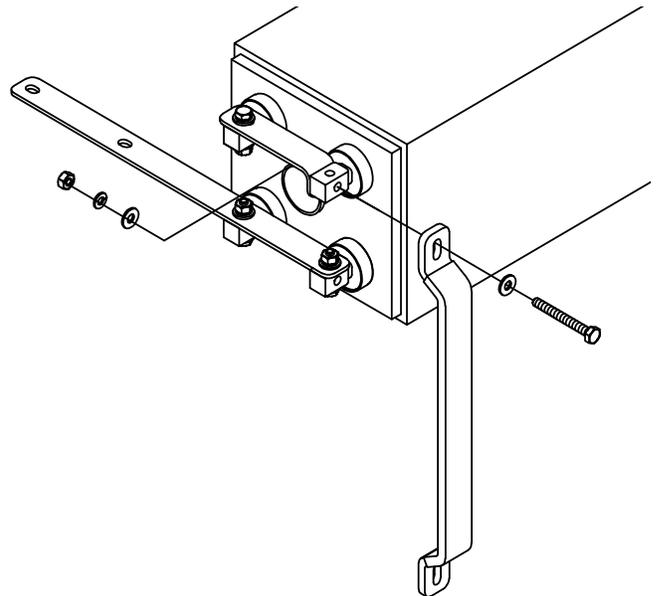
3. Ensure proper alignment of connectors to cell posts.
