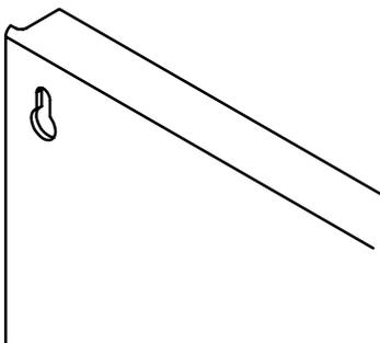
3. One shield will cover two modules. Starting at the bottom of the stack; hang the first shield on the top brackets through the large part of the keyhole. At the same time aligning the cutout at the bottom of the shield with the second set of brackets. The next shield will overlap the previously installed shield. For stacks containing odd number of modules a single module safety shield will be supplied. After all shields are in place, tighten the outer bolt, but **do not torque**.
