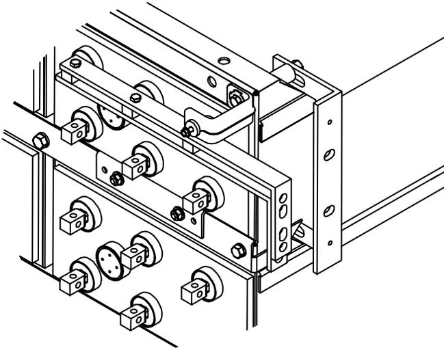
5. Install side terminal plate to terminal plate bracket using 1/4-20 x 1.00" hardware. Bolts should be installed loosely for future adjustments.
