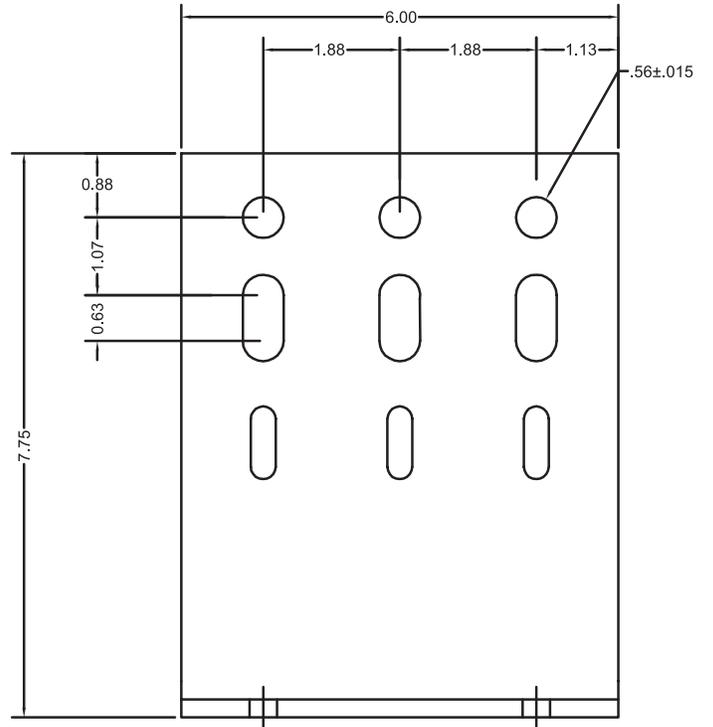
Top terminal plate hole to hole dimensions typical.
