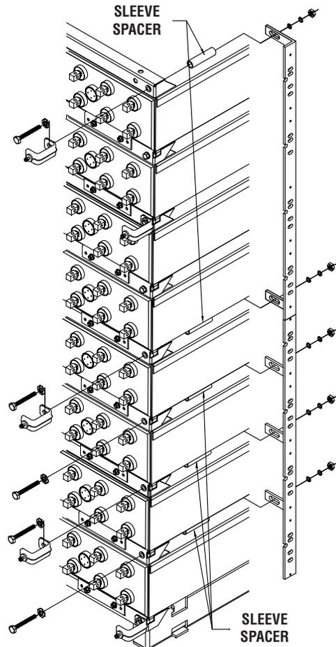
10. Side terminal plate is designed to use up to 0.50" dia. bolt and a maximum 1.75" centers, 2 hole lug. Plate is capable of handling 4 runs of cable. Lugs can be positioned on both sides of the terminal plate. **Lug and lug hardware not included.**
