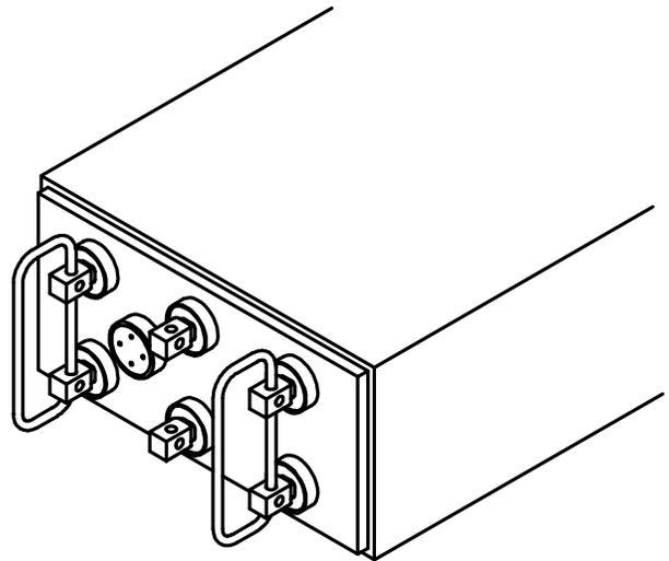
8. Pull cell from module onto lifting device. Care should be taken so lifting device does not come in contact with cell posts.
