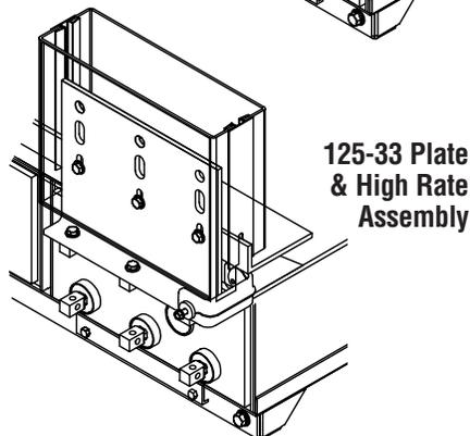
8. Top terminal plates are designed to accept up to 0.50" dia. bolt and use a maximum 1.75" center, 2 hole lug. **Lug and lug hardware not included.**
