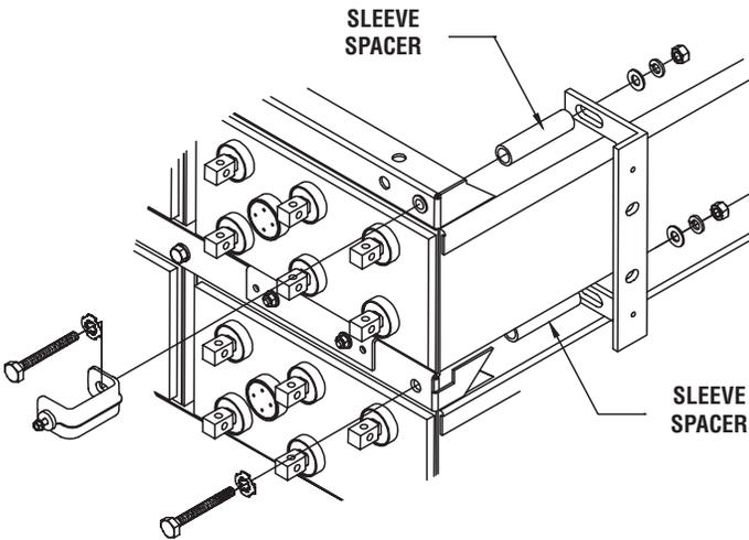
3. The side terminal may be located at the bottom module. Slot in lower arm of side terminal bracket slips over tab in base plate. The upper side terminal bracket connection should be attached as called out in previous section.
