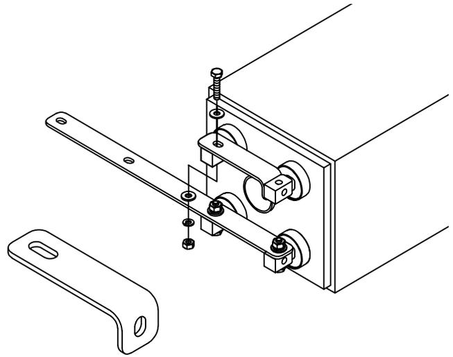
2. Install “C” connector to cell post using horizontal bolt as below. Bolt should be installed loosely for future adjustments. Duplicate connection process at both connection points.
