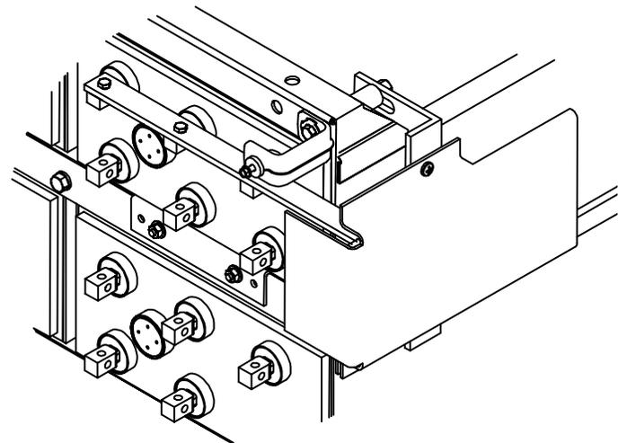
9. Depending on the termination location, side terminal plates may be adjacent to each other. The side terminal bracket attachment is different depending on the number of adjacent terminal plates.
