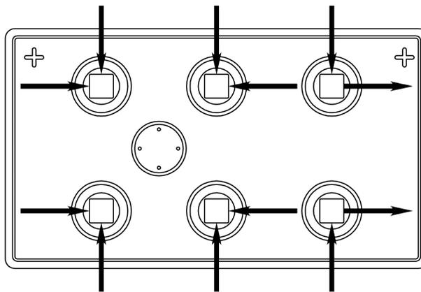
4. Unigy II battery strings are typically supplied with connector package 1CU requiring one connector per post.
