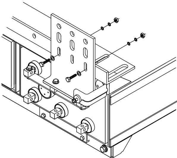
6. Assemble the four parts of the top terminal safety shield as detailed below.
