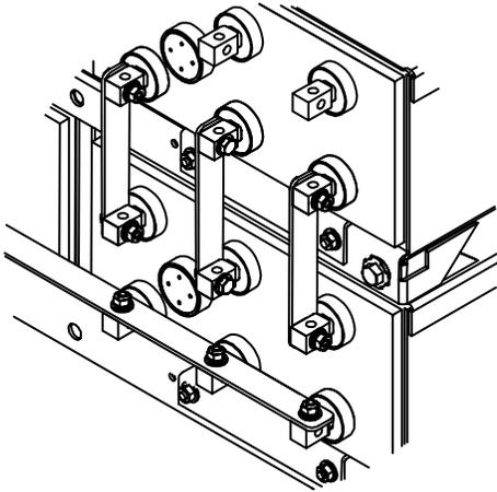
5. High rate applications will require multiple connectors to be used per cell post. A 2CU connector package will require 2 connectors per connection (1 per side), see example below. A 4CU package will require 4 connectors per connection (2 per side) and a 6CU package will require 6 connectors per connection (3 per side). Tighten & torque all bolts after all connectors are installed. Consult "Hardware Torque Requirements" (pg b.4) for proper torque values.
