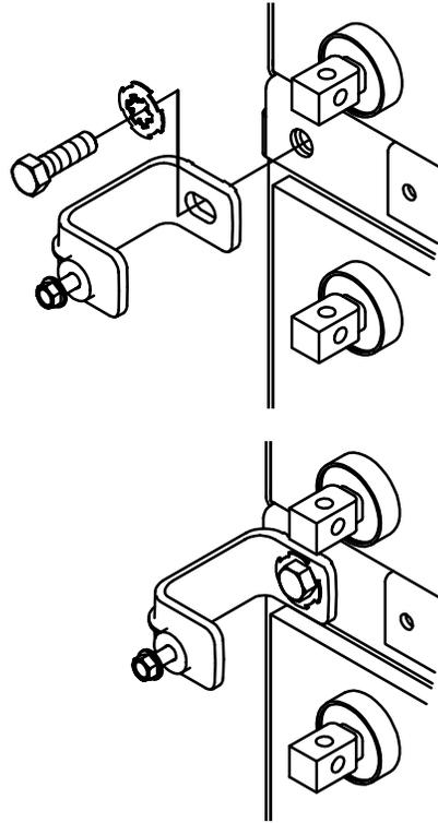
10. Module layout should be compared to battery string layout diagram and all hardware should be checked for proper torque before proceeding. Consult "Hardware Torque Requirements" (pg b.4) for proper torque values.
