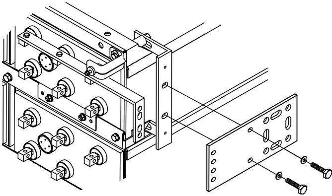
6. Connect side terminal plate to side terminal plate connectors. Bolt length is dependent on connector package as noted below.
