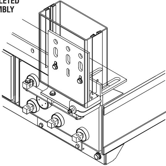
7. Top terminal assembly will vary by battery plate size.
