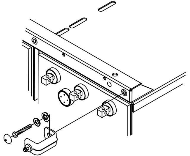
2. Install terminal plate bracket to the top of the module. Use 3/8-16 x 1.25" hardware. Install loosely for future alignment.
