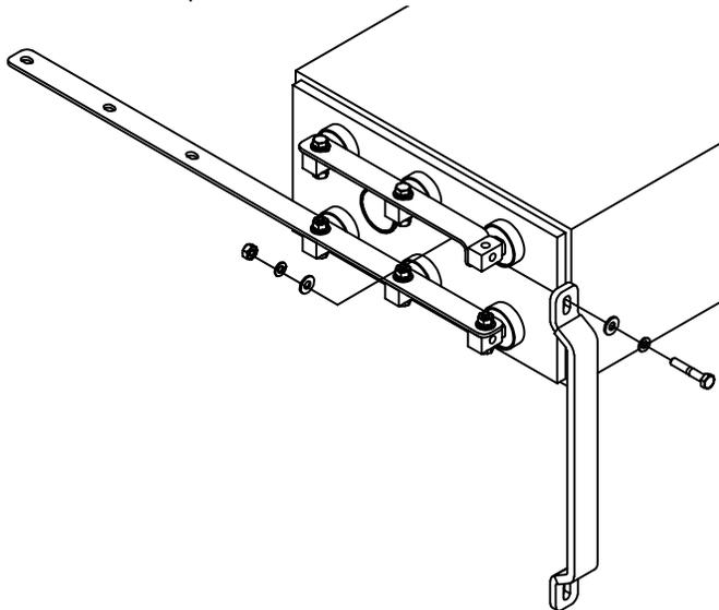
3. Ensure proper alignment of connectors to cell posts.
