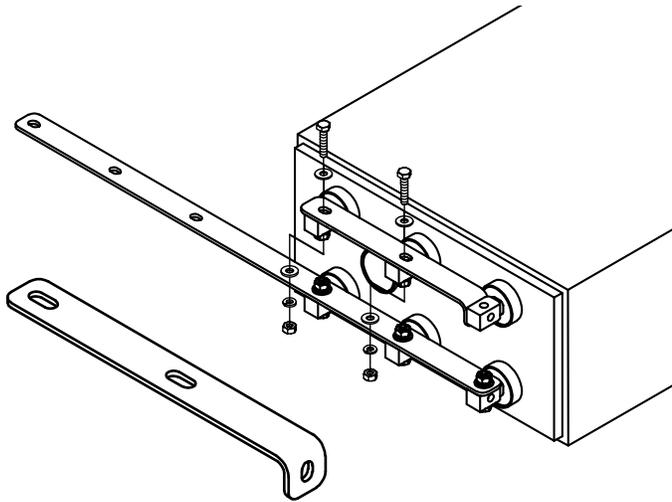
2. Install "C" connector to cell post using horizontal bolt as below. Bolt should be installed loosely for future adjustments. Duplicate connection process at both connection points.
