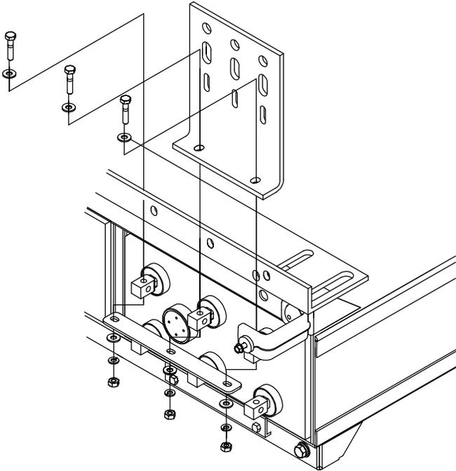
5. After confirming alignment safety shield bracket hardware should be tightened, but not torqued. All remaining hardware should be torqued. Consult "Hardware Torque Requirements" (pg. b.4) for proper torque values.
