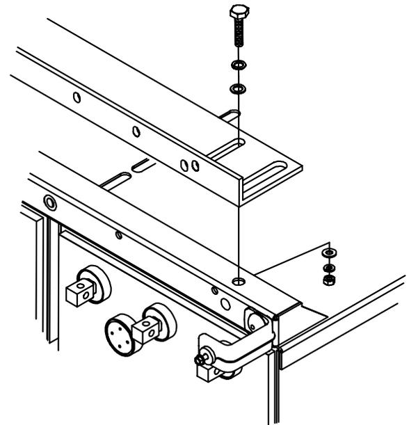
3. Install terminal plate to battery posts using 1/4-20 hardware (consult battery string layout diagram & parts kit for specific length).
