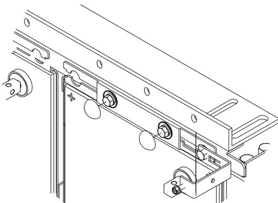
5. Install terminal plate to battery posts using 1/4-20 x 1.00" hardware.
