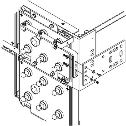
5. Connect side terminal plate to terminal plate bracket using 1/4-20 x 1.00" hardware. Bolts should be installed loosely for future adjustments.
