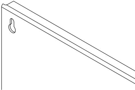
3. One shield will cover one module or two tiers. Starting with the bottom module, hang the first shield on the top brackets through the large part of the keyhole. At the same time aligning the cutout at the bottom of the shield with the second set of brackets. After all shields are in place tighten, but **do not torque** hardware.
