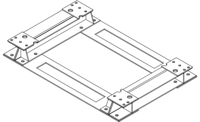
3. Multiple stack systems should have a minimum of 4.00" between bases. The additional spacing is for proper installation of modules.
