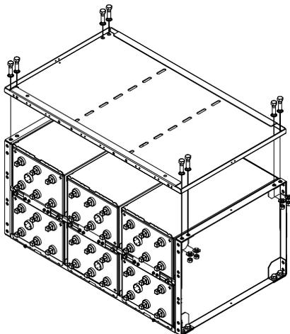
Star washers are to be installed with teeth towards module to ensure proper grounding.
