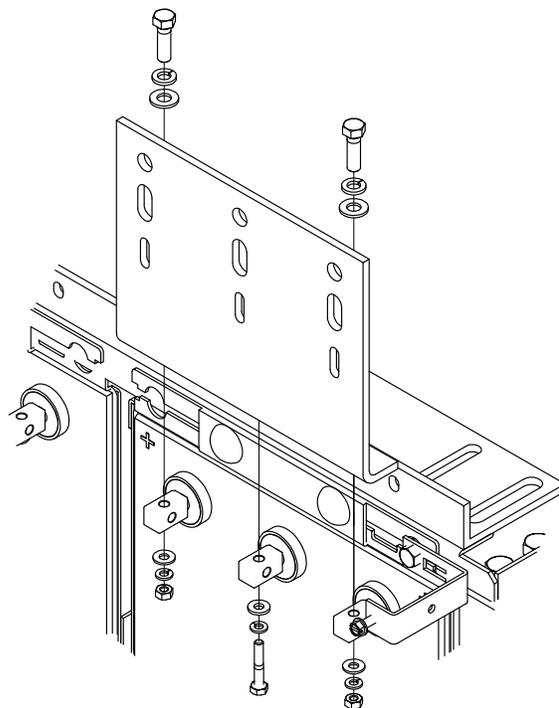
**Terminal Plate to be installed on battery posts as shown**
