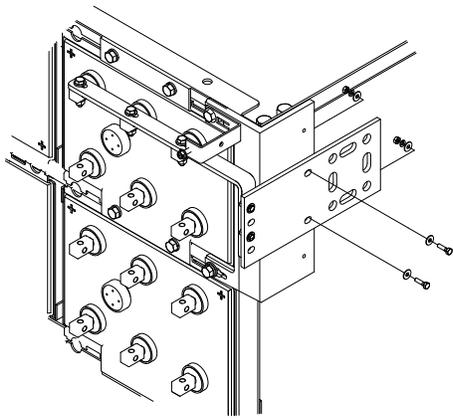
6. After all parts are installed and alignment is confirmed, torque all bolts. Consult "Hardware Torque Requirements" (pg 5) for proper torque values.
