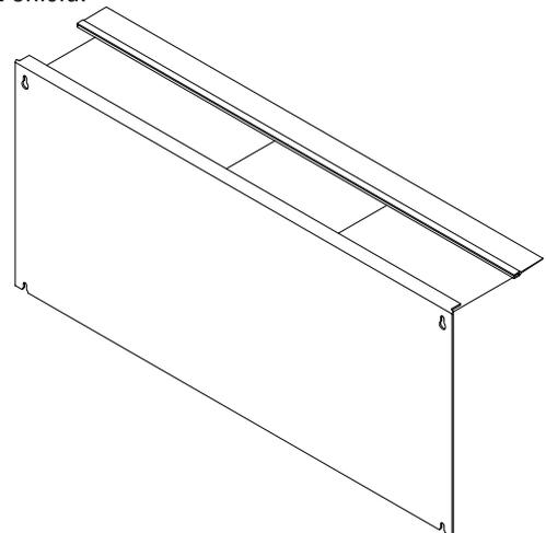
For top terminal assembly, align protective cover in front of top terminal plates. Mark area of protective shield that is required to be removed in order to fit between the terminals. Cut protective cover along marks.
