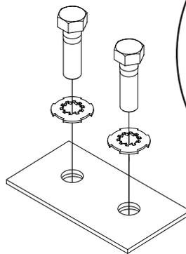
8. Bolt assemblies (two per corner) are required on the outside of the module to complete the base to module connection. All ½-13 x 1.75" hardware should be checked for proper torque before proceeding. Star washers are to be installed with teeth towards module to ensure proper grounding. **Consult "Hardware Torque Requirements" (pg 5) for proper torque values.**
