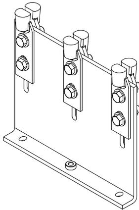
10. **Safety Shield Installation** — Top terminal safety shield consists of three pieces. Assemble per the below illustration. Clear plastic shields are of different lengths. Longer shield to be installed on the front side of the terminal plate. The shields should be even at the bottom, making the front shield longer at the top.
