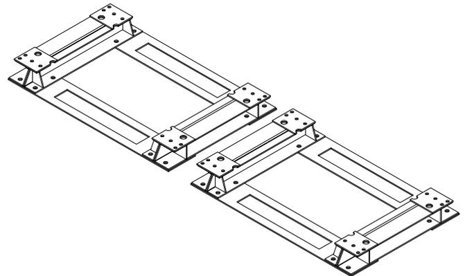
4. Anchor holes can be marked and drilled with bases in place. All anchor holes in base (16 per base) are required to be used to meet NEBS Zone 4 seismic requirements. Anchors required to be installed prior to modules being installed onto base. Reference Appendix A for base plate anchor hole layout.
