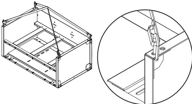
7. Base and module layout should be compared to system layout diagram. All 1/2-13 x 1.75" hardware (2 per corner) are to be installed on the inside of the module for module to base connection. All hardware should be checked for proper torque before proceeding. Star washers are to be installed with teeth towards module to ensure proper grounding. Consult "Hardware Torque Requirements" (pg 5) for proper torque values.
