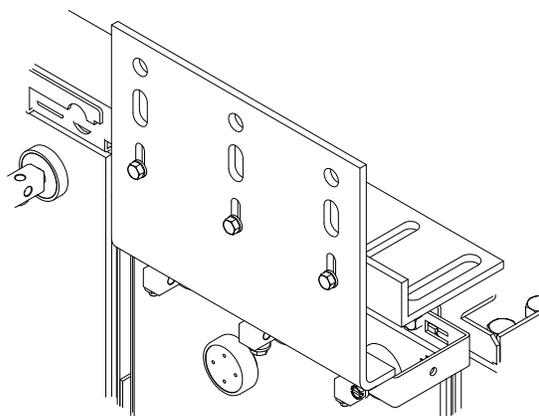
8. **Lug Hole Layout** — Top terminal plate designed to use up to 0.50" dia. bolt and a maximum 1.75" centers and 1.188" min., 2 hole lug.
