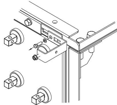
2. Install plastic Side Terminal Bracket and re-install safety shield bracket using bolts from previous step. Use 3/8-16 x 1.50" bolt for the remaining bracket assembly. Bolts should be installed loosely for future adjustments.
