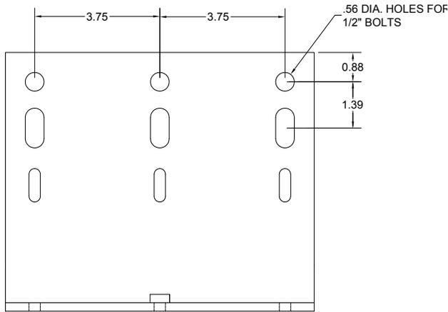
9. **Lug Attachment** — Maximum of six cable lugs can be installed per terminal plate. Lug Hardware not included.
