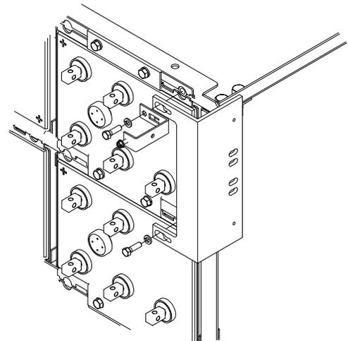
3. Install side terminal connector to battery posts using 1/4-20 hardware plate to terminal plate bracket using 1/4-20 x 1.00" hardware. Bolts should be installed loosely for future adjustments.
