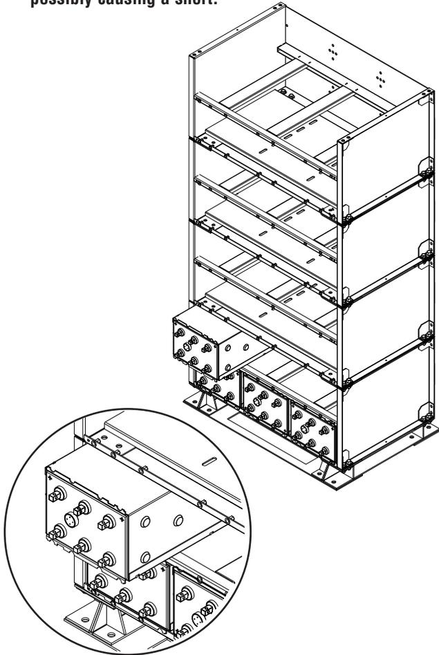
12. **Top Plate Installation** — The top plate is to be installed on the top module after all cell / sleeve assemblies have been installed. Bolt assemblies (two per corner) are required on the outside of the module to complete the top plate to module connection. All 1/2-13 x 1.75" hardware should be checked for proper torque before proceeding. **Consult "Hardware Torque Requirements" (pg 5) for proper torque values.**
