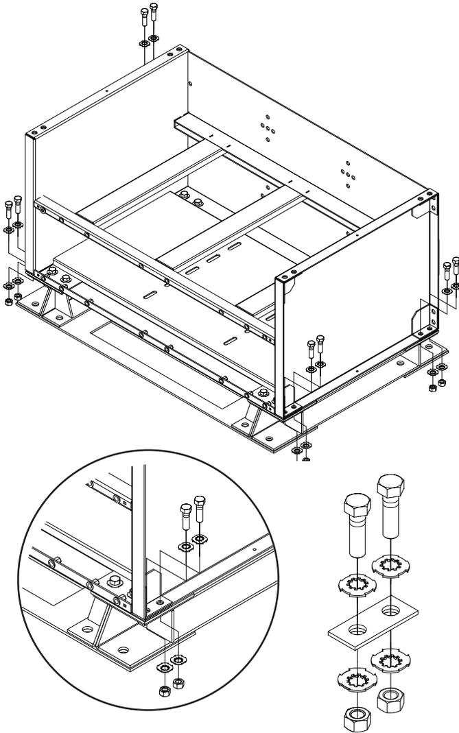
9. **Multiple battery systems** — all stacks should have the same tier completed before moving to the next tier.
