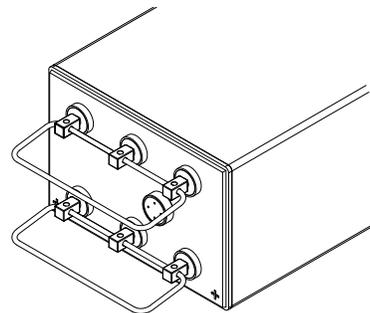
8. Remove the two retaining bars holding in the cell to be removed.
