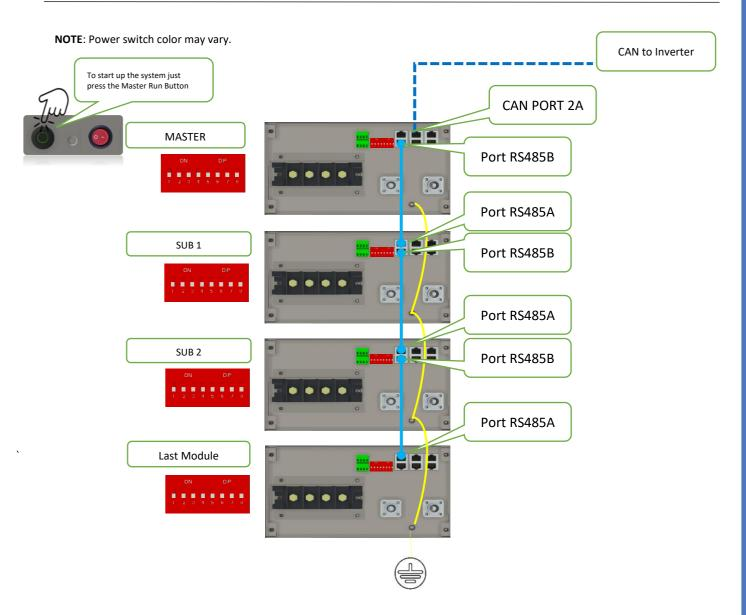
2.5.1 Auto ID Assignment and DIP Configuration for LOW Voltage Single Cluster (Parallel Connection)
