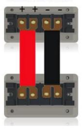
The low voltage screw terminal only supports parallel connection with maximum voltage 60V CAUTION> Connecting these terminals in series will cause serious damage to the battery
