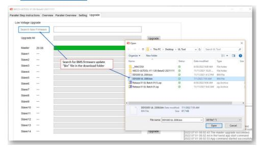
Make sure that the connection between the battery converter and the PC is stable for the duration of the update process. Do not disconnect the connection before the software has confirmed the upgrade. Click OK.
