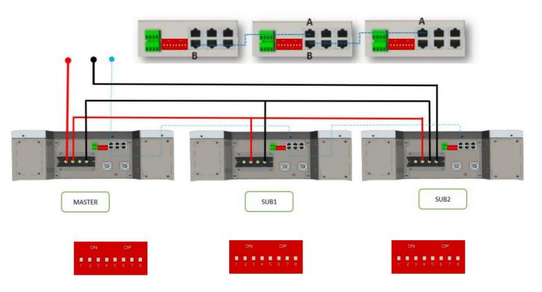
Note: In a single cluster configuration, there is no need to set the DIP switch on the master battery. All DIP switches should be set to OFF. The single cluster will self-configure.
