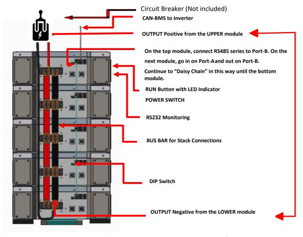
Note: The Run Button, Power Switch and RS232 Port are located on the right side when facing the unit. Deka label on the top.
