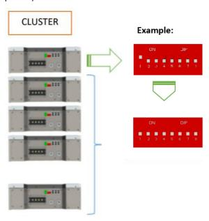
The First Battery of the cluster after being set with the ID (acting on the DIP switches) will auto assign all the sub Module addressees.
