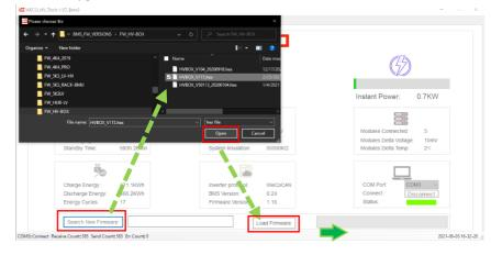
After confirming the File and clicking on the LOAD FIRMWARE button, the update procedure will begin and the HV BOX will be updated to the latest version.
