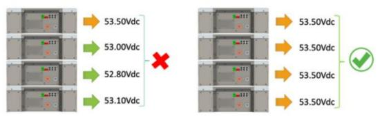
It's recommended to individually charge all modules at the same level before proceeding with the final installation
