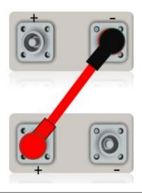
Fast Connector terminals only support series connections up to 1000Vdc
