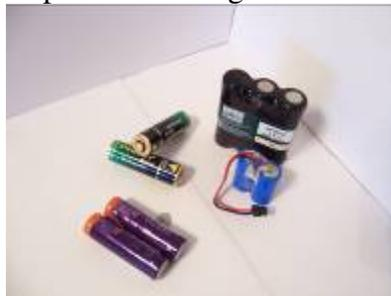
Shrink-wrap – A plastic material covering the majority of the exterior of the cell configuration or pack that is heat-formed, causing the plastic material to shrink and form tightly around the contents. These battery packs will also have terminations that could be one of the following: pressure contact, bare leads or a plug-type termination.
