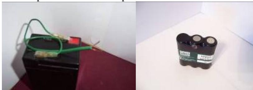
Cut off wire leads flush or cover leads and or pressure contacts with tape or some other non-conductive material to prevent short circuit hazards.
